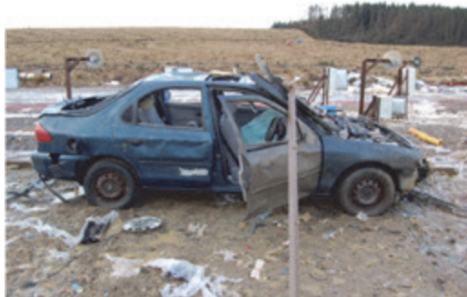
(f) Test 4.2-4 Car 1 at 6 m – overpressure 3428 mbar (shock)
