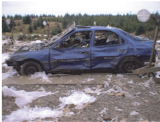
(b) Test 4.2-2 Car 1 at 6 m – overpressure 11050 mbar (Max), 5191 mbar (shock)
