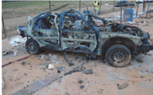
(a) Two views of Ford Mondeo car damaged within the cloud in Test 4.2-1
