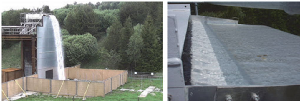
Figure 3.1 Liquid spills facility at HSL (Buxton) showing Test 1 in progress (left) and the 1500 mm wide chute projecting 400 mm from the tank wall (right)
