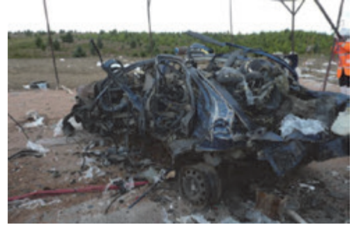
(a) Two views of Ford Mondeo car damaged within the cloud in Test 4.2-1
