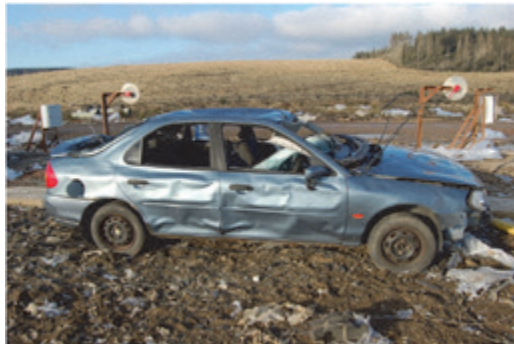
(d) Test 4.2-3 Car 1 at 6 m – overpressure 5209 mbar (shock)
