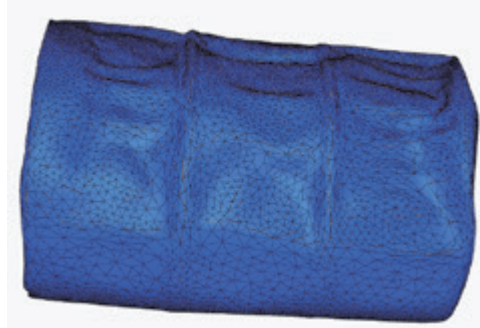
(a) 90% full oil drum on its side inside the gas cloud in Test 4.2-4
