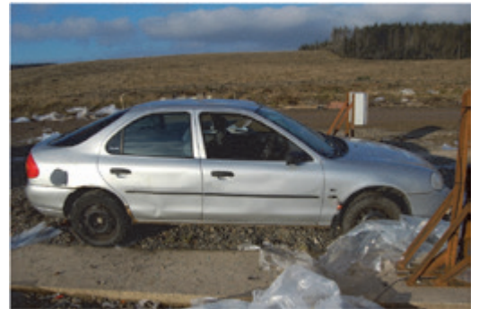
(e) Test 4.2-3 Car 2 at 15 m – overpressure 1074 mbar (Max), 693 mbar (shock)
