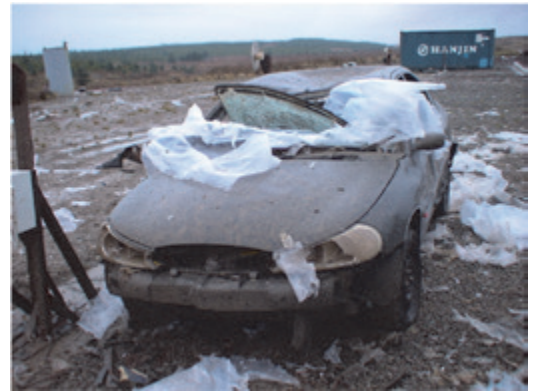
(c) Test 4.2-2 Car 2 at 15 m – overpressure 1211 mbar (Max), 1126 mbar (shock)
