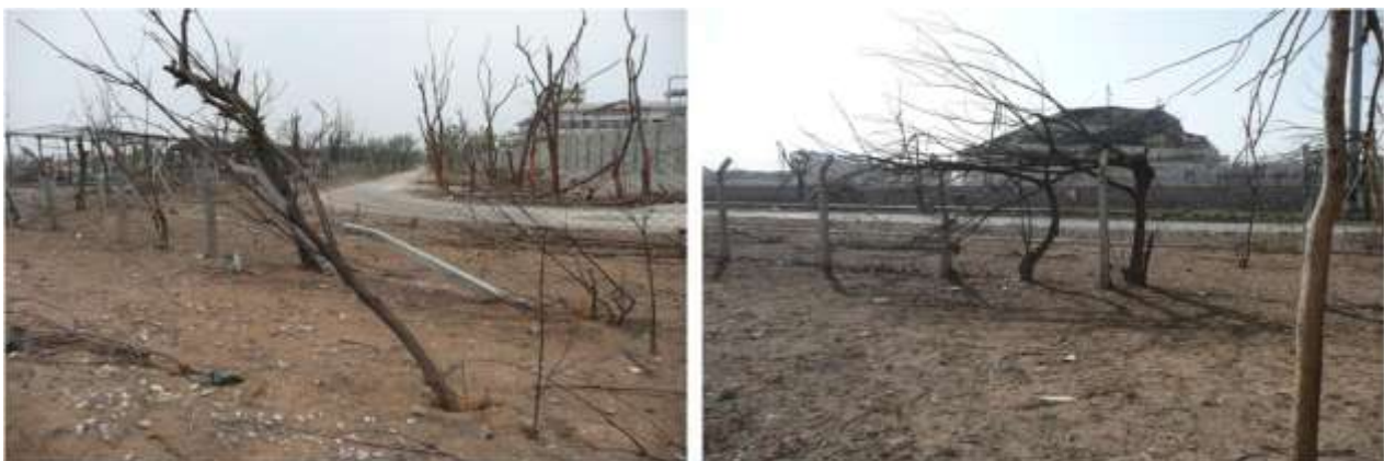
Figure 30: Directional indication provided by trees in the main tank area
