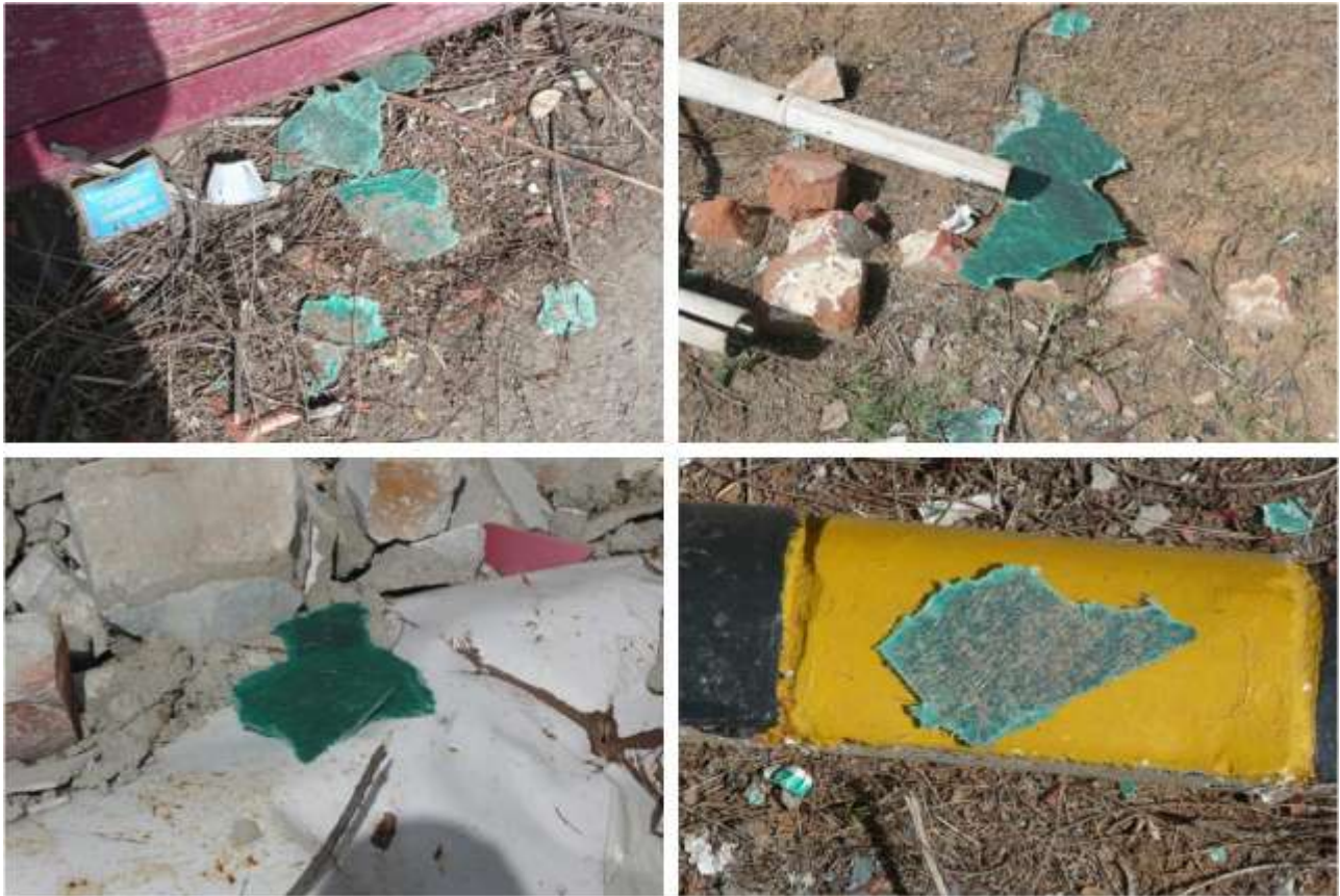
Figure 18: Broken pieces of the fibreglass sheet
