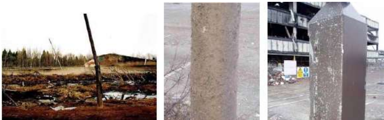
Figure 82: Directional indicators inside the Buncefield cloud
