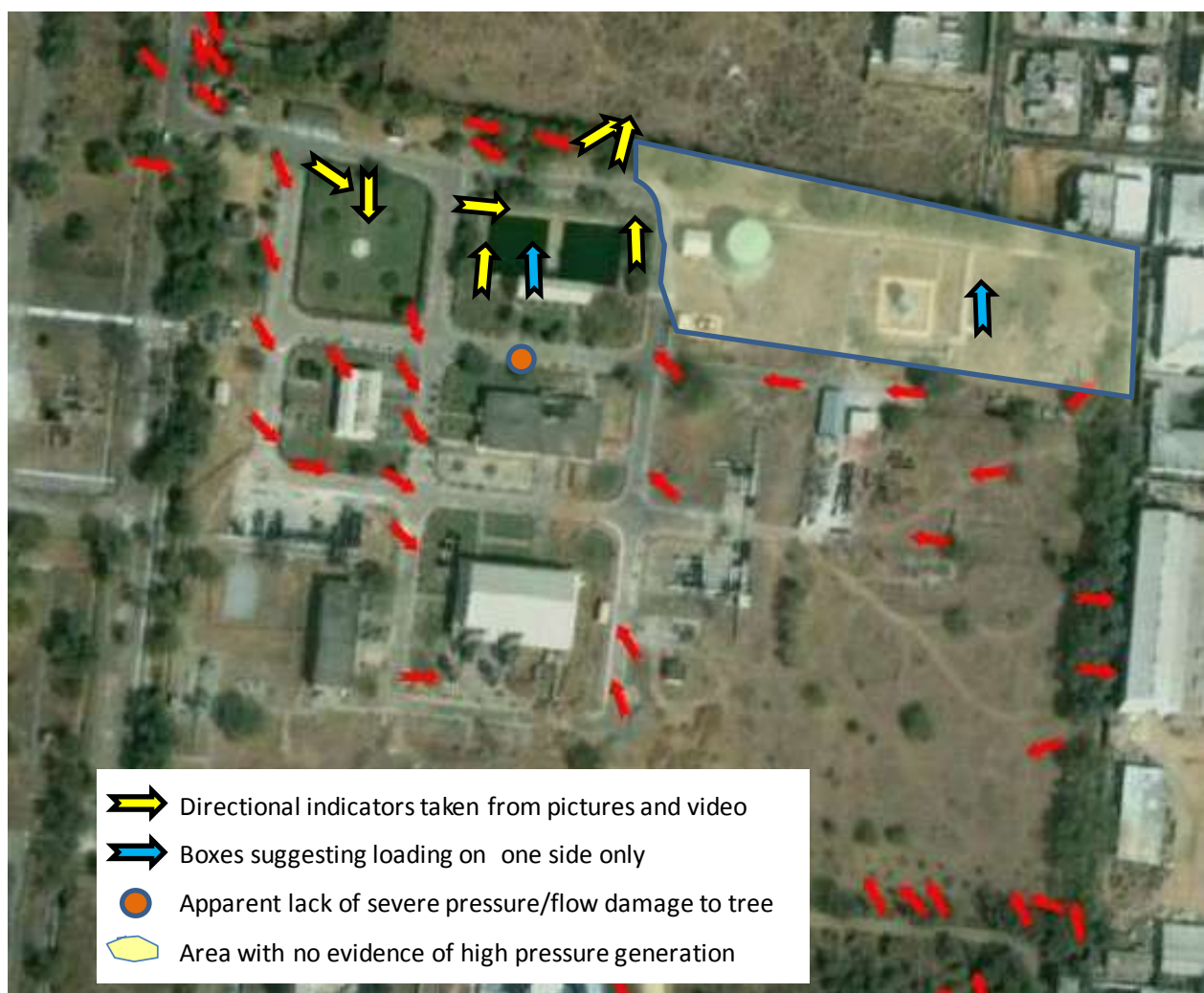
Figure 7: Directional indicators in the Pipeline Division area and area without apparent pressure generation
