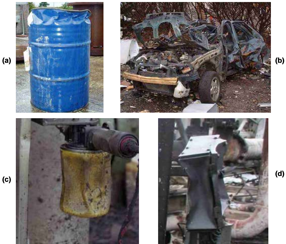
Figure 80: Examples of the types of pressure damage observed within the Buncefield cloud; (a) Damage to near full steel drum in static test; (b) Damage to car; (c) Crushing of oil filter; (d) Crushing of steel box
