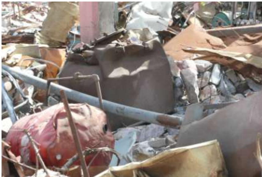
Figure 15: Crushing of tank and steel drum
