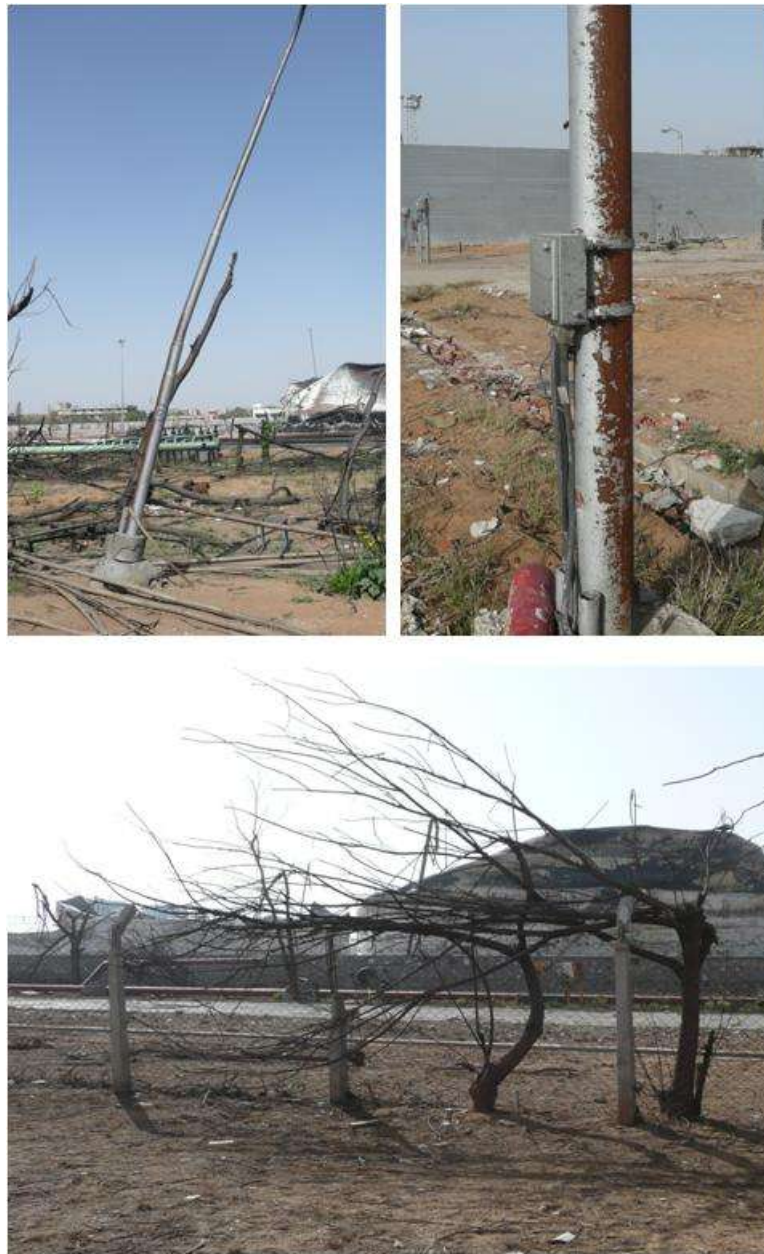
Figure 5: Example of directional indicators
