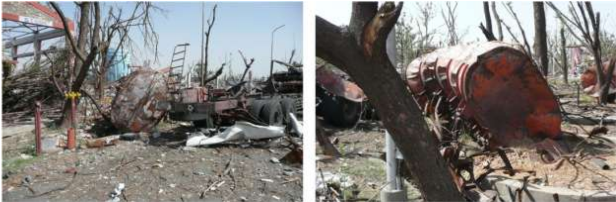
Figure 14: Road tanker with tank displaced and crushed
