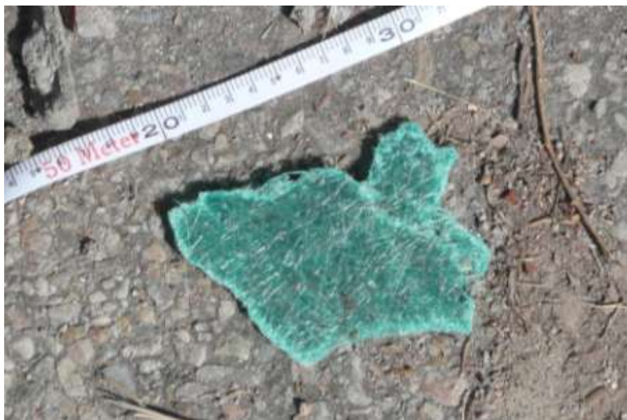
Figure 19: Single piece of diamond shaped fibreglass sheet (note fracture line along irregular edge)
