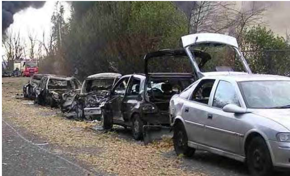
Figure 81: Change in Damage Level to Cars at the Cloud Boundary
